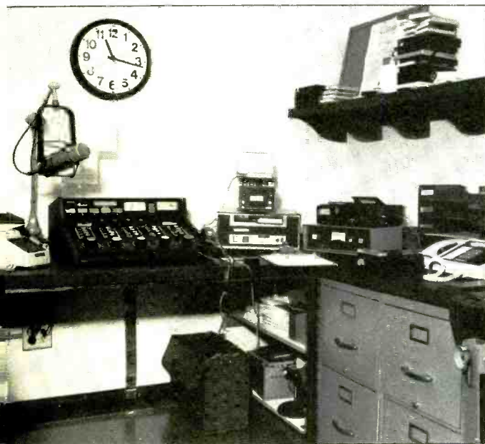
In newsroom, all news is gathered, edited, and put on the air. Control console is center rear. Other units: cart players, reel-to-reel machines, weather equipment, cassette player
