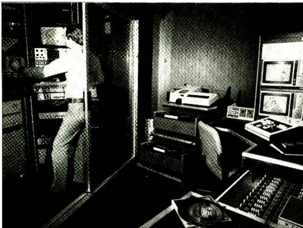
The Sausalito facility includes EC 103B edit controllers and Sony one-inch and 3/4-inch videotape recorders
