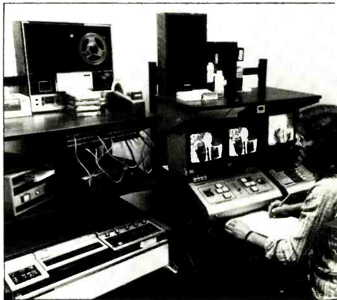
The four ENG edit booths are adjacent to both the newsroom and production control. The VCR playbacks are also located close to the edit booths
