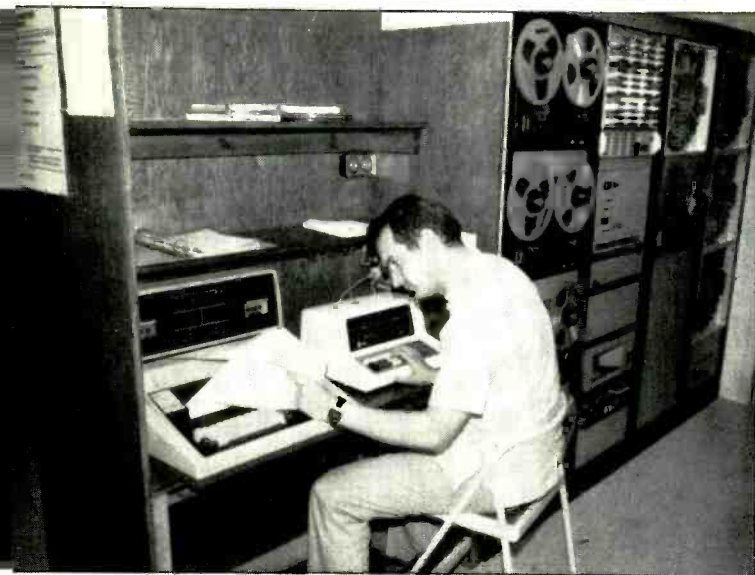
Richard Sweetland, general manager, sets up programming at input to automation system, which is to his right. Harris System 90 includes four music tape decks, an Instacart, four carousels
