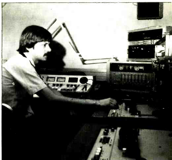
Production room has reel-to-reel recorders, turntables, cart machines around operator. Audio processing equipment is just to rear right of console
