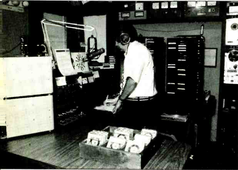
Main control room is all-stereo, to be ready for AM stereo. Equipment can be used in standup operation; most music is on carts. Program director Gary Jackson conducts air show
